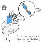
Once battery is removed, gently disconnect battery connector; do not pull hard.
