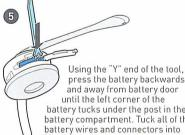
press the battery backwards and away from battery door until the left corner of the battery tucks under the post in the battery compartment. Tuck all of the battery wires and connectors into the battery compartment.
